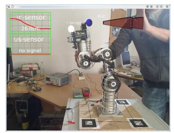
(a) Visualization for engineers, presenting the current measurement of the two sensors
